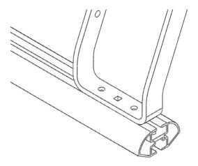
Align the round tabs on the bottom of the wheel holder so that they rest in the top slot of the load bar.
