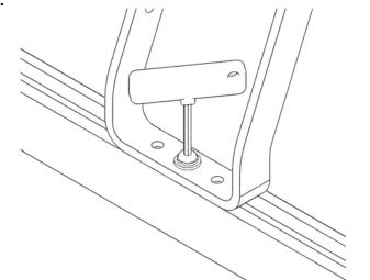
Loosely tighten the button head screw with the hex key.
