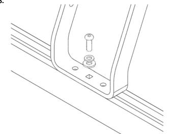
Place the flat washer on top surface of the wheel holder.
