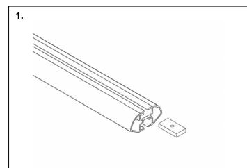
Remove the end cap from the load bar by loosening the narrow shoulder hex screw.
