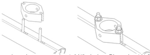
Place the tube adaptor over the 1-3/4" t-bolts. Place the 1/4 flat washers and loosely tighten 1/4-20 lock nuts onto the 1-3/4" T-bolts. Repeat for the other tube adaptor.
