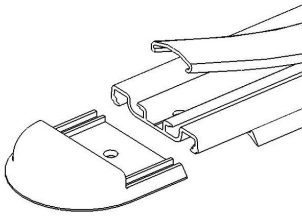
Center the bottom gasket on each track by sliding the end caps into the ends of the track.
