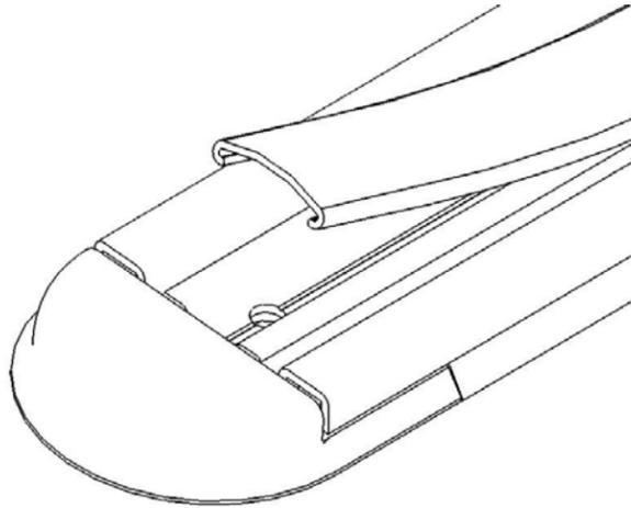
Temporarily secure the end caps to the track with tape. Lift the edges of the top gasket enough to reveal both corner holes.
