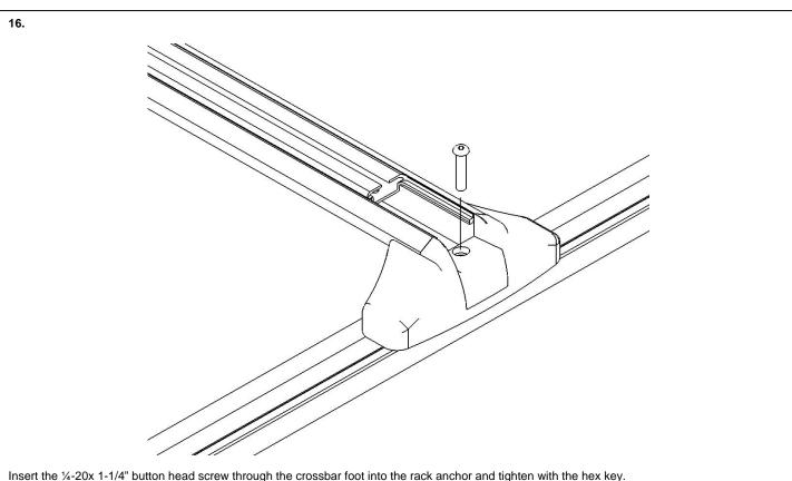
insert the %-20x 1-1/4 button head screw through the crossbar loot into the rack anchor and tighten with the nex key.
