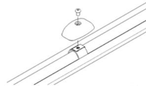
Install the crossbar anchor covers using 1/4-20 X 3/8" button head screws.
