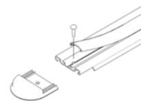
Pull back the top track cover at each end. Slide the end caps on and secure by using the remaining drill screws.
