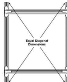
Ensure that the assembly is square by taking diagonal measurements from corner to corner. When the measurements are equal, fully tighten the crossbars to the tracks. Place the assembly on the roof and position using the suggested dimensions in step 5.
