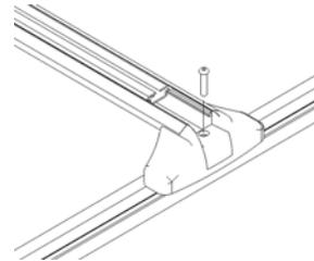
This step is performed on a workbench or floor, not on a vehicle. Lay the tracks side by side with the raised rib sides of the anchors facing each other. Use a crossbar kit or template to correctly space the tracks. Using 1/4"-20 X 1-1/4" button head screws (supplied with crossbars) secure each crossbar through an anchor to the track. Crossbars are used only to position the track and will be removed later.
