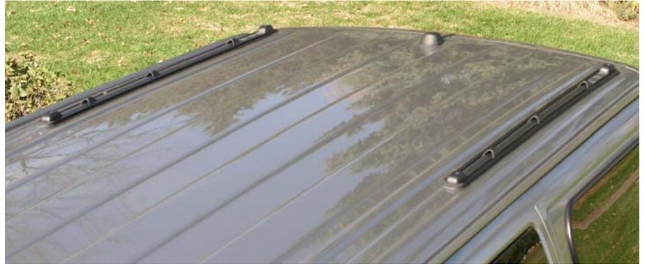
**Note:** For proper width placement of roof tracks, an optional crossbar template or roof rack crossbar kit should be used for installation.
