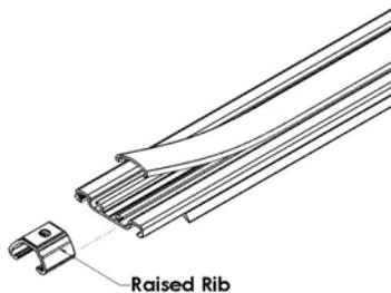
Remove the top gasket on each track. Slide two crossbar anchors onto each track. The sides marked with the raised ribs should face each other.
