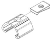
Attach U-clips to the four sliding anchors. ⚠ Make certain the u-clips are oriented as shown.
