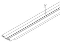
Center the bottom gasket on each track (approx. 1-3/16" from each end). Reposition the tracks on the roof over the punch markings. Attach the tracks to the roof using drill screws in all mounting holes **except the end positions**. Silicone can be used to prevent leaking.
