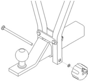
Slide the carriage bolt through the square cutouts beneath the clamp jaws. Place the washer onto the carriage bolt and screw the locking knob onto the carriage bolt.
