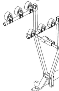
Squeeze handle and push down on center of handle until handle locks into place.
