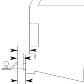
Ball mount must be inserted into receiver and have a minimum of 2 -1/2 inches from the rear of the vehicle to the ball mount drop.
